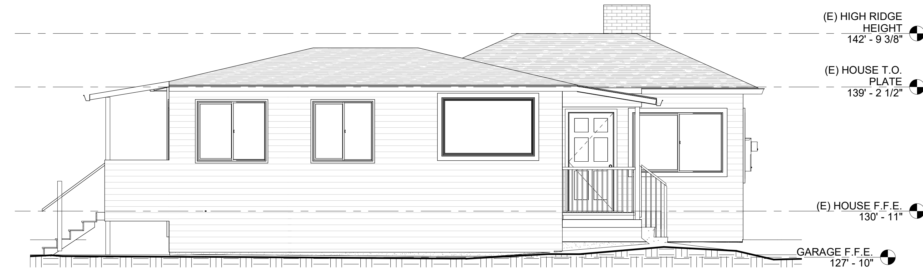
② EXISTING LEFT SIDE ELEVATION 1/4" = 1'-0"
