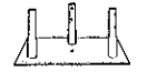
CONCRETE BASE PLATE - RUC 25GP FOR USE WITH ANY Rohn 25G GUYED TOWER STRUCTURE. Additional base information available please see page 18.
